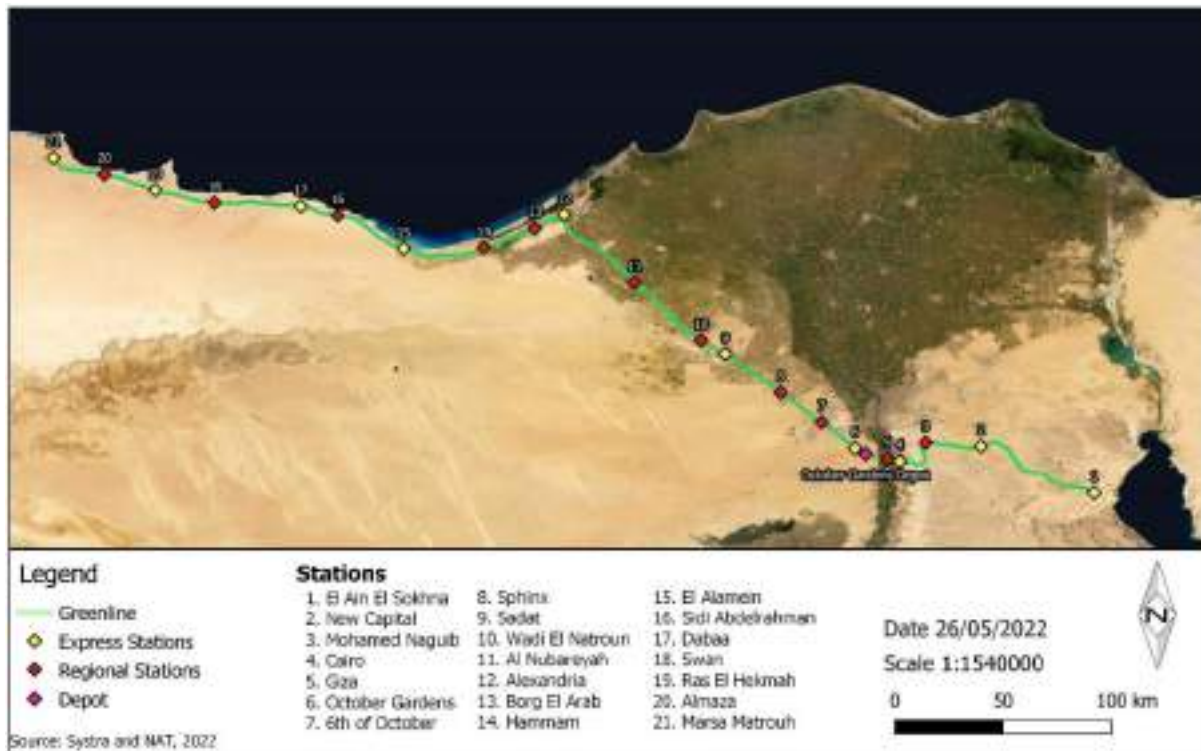
Figure 2-1 HSR Green Line Alignment
