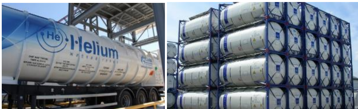
Figure 4.18: Isothermal tanks for liquefied helium transportation 29
